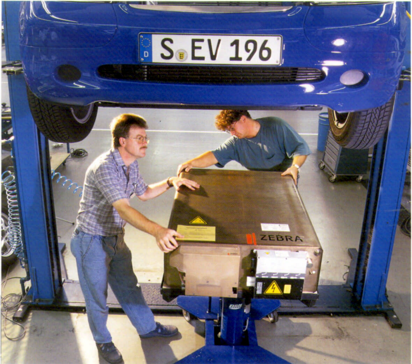
Putting it together: The complete ZEBRA battery block is fitted into the A-class EV from below.
