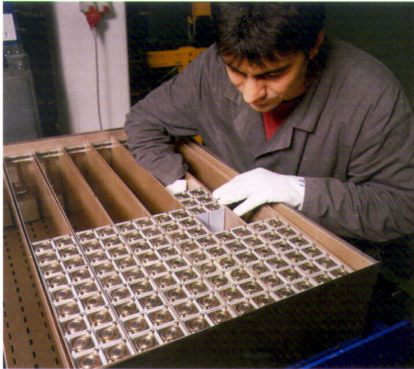
Packing in the power: The ZEBRA battery block in the A-class EV consists of 448 individual cells.
